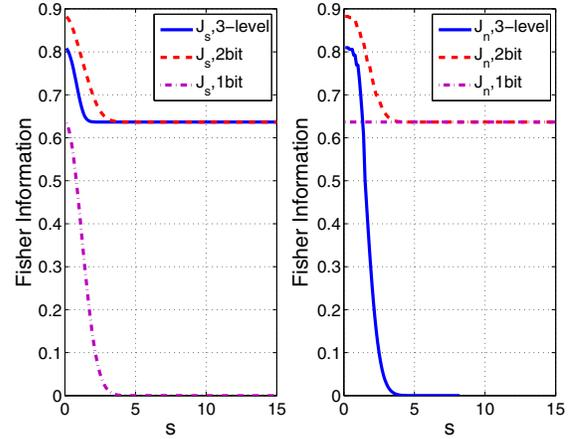
Fig. 1. Fisher information of signal ( $J_s$ ) and noise ( $J_n$ ) for 1bit, 2bit and 3-level quantization under different signal  $s$  ( $\sigma = 1$ ).
