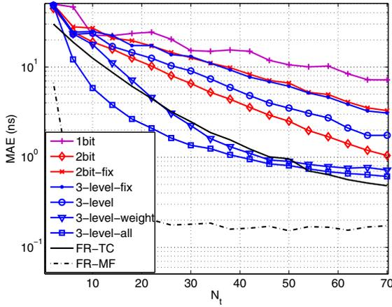
Fig. 2. MAE of TOA estimation using quantized samples for different receivers vs. accumulation period  $N_t$  ( $E_b/N_0 = 12dB$ ).
