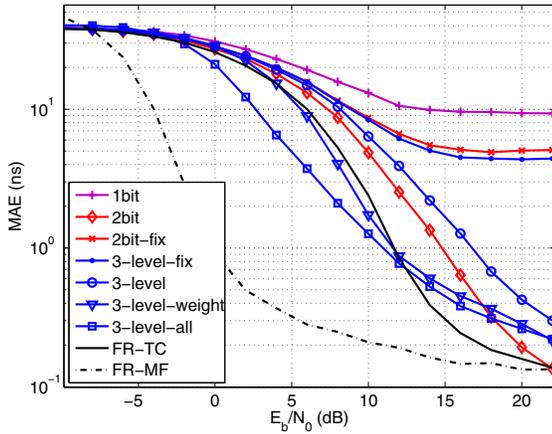
Fig. 3. MAE of TOA estimation for different sampling receiver under CM1 vs.  $E_b/N_0$  ( $N_t = 50$ ).
